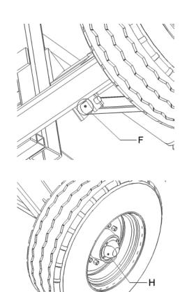
Grease wheel bearings (H) sparingly – six "shots" of grease every 150 hours.
