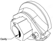
Unbolt and remove the nut locks from the end washers on both ends of the axle.
