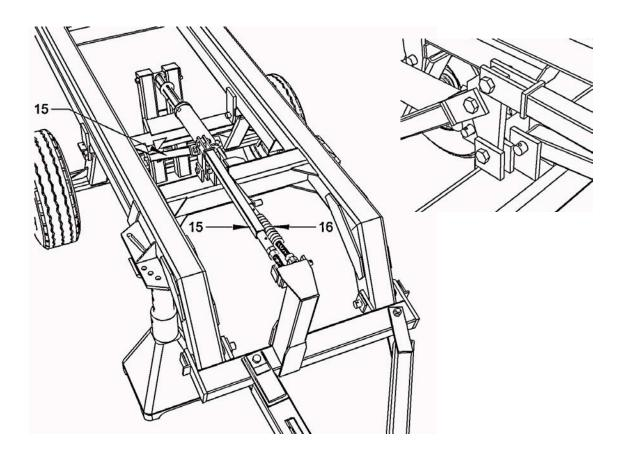
17. It is now possible to lift the hitch of the disk and remove the support from under the frame. Leave the tire chocks in place. At this point the hydraulic hoses can be connected to the cylinder but do not charge the system.
