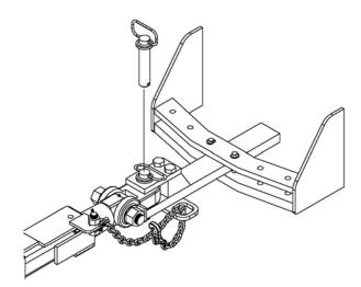
Install the drawbar pin and its retaining hardware. This may require moving the tractor forward or backward slightly. An articulated tractor or belted tractor can swing the drawbar side to side by turning the steering wheel slightly. This procedure may take more than one attempt – safety takes time.
