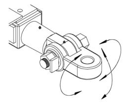
The disk is equipped with a heavy tongue that both flexes and swivels to accommodate the most rugged terrain including large rocks and tree stumps. This is an essential design feature; however it requires extra care when attaching the disk to a tractor.
