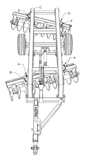
To change the angle of the front gang, loosen the bolts at positions A and remove the bolt at position B. With the disk slightly lowered into the ground, use the tractor to carefully move the disk either forward or backwards to the desired position. Reinstall bolt B and tighten all four bolts to 1500 ft/lbs.
