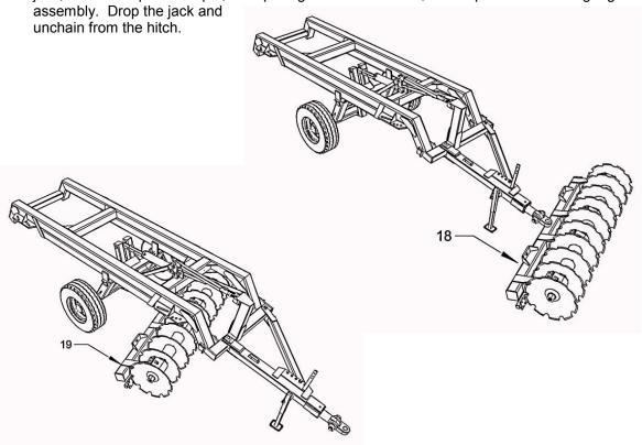
20. Using a single strap or chain of sufficient strength wraped around the center balance point of the gang bar, lift straight up throught the frame. This may require fork extensions or a boomlift. Once a single bolt and nut is installed (do not tighten), the gang bar assembly may
